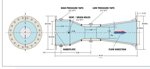
**Liquid Applications**: All impulse piping must have minimum 1 inch per foot, DOWN to the flow transmitter(s). Transmitter at or below the meter center line.
