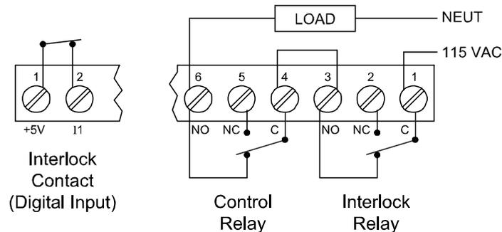
Figure 18. Interlock Connections
