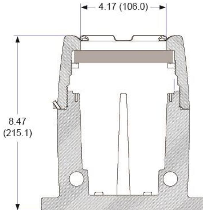
Figure 24: Enclosure Dimensions – Side Cross Section View
