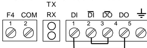
Figure 10. Three-Wire RS485 Connection
