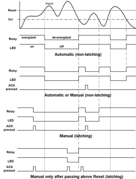
For Manual reset mode, ACK can be pressed anytime to turn "off" relay. For relay to turn back "on", signal must go above set point and then go below it.
