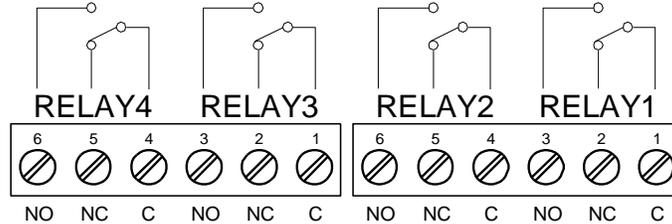
Figure 13. Relay Connections
