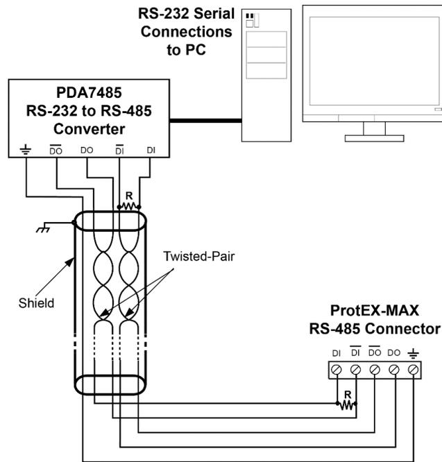
Figure 11: RS-485 Wiring
