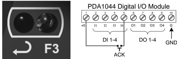
Figure 20. Acknowledge Relays w/Function Key or Digital Input
