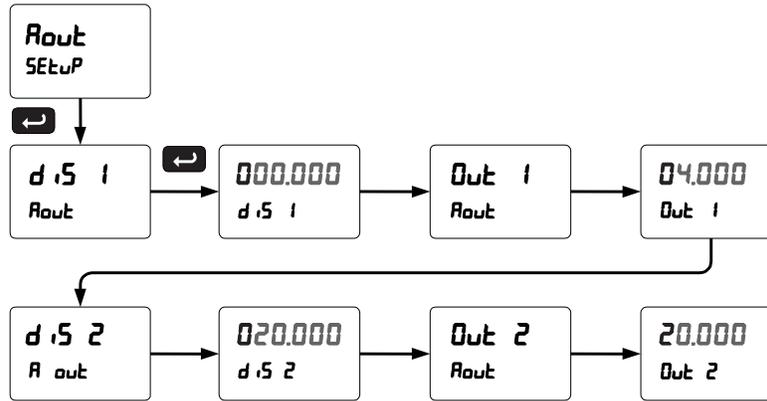
*Note: During the analog output scaling, the display value is always indicated with a decimal point regardless of the decimal point selection for the temperature display.*
