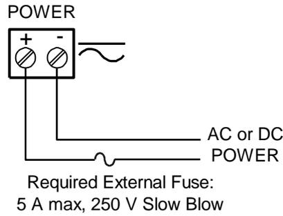
**Figure 3. Power Connections**
