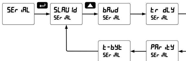
When using more than one meter in a multi-drop mode, each meter must have its own unique Slave ID or meter address. The ID or address may be programmed between 1 and 247. The transmit delay may be set between 0 and 199 ms. The parity can be set to even, odd, or none with 1 or 2 stop bits.
