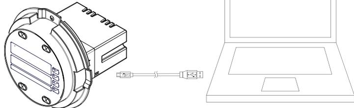
2. Once the driver is installed, an AutoPlay dialog should appear for the drive "MAINSTAL." Click "Open folder to view files." If the computer does not display an AutoPlay dialog for the drive "MAINSTAL," you should open My Computer and double-click on the drive labeled "MAINSTAL."
