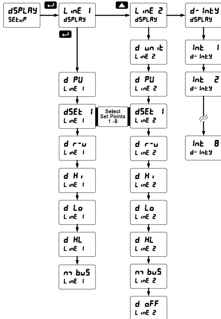
**Display Intensity:** The meter has eight display intensity levels to give the best performance under various lighting conditions. Select intensity 8 for outdoor applications. The default intensity is 8.
