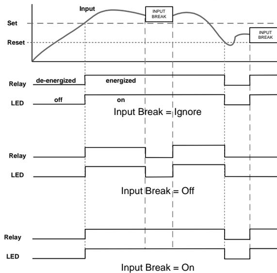
When the meter detects a break in the input, the relay will go to one of the following selected actions:
