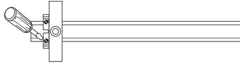
2. Assemble the two parallel mounting rods using cross rods provided with modules.
