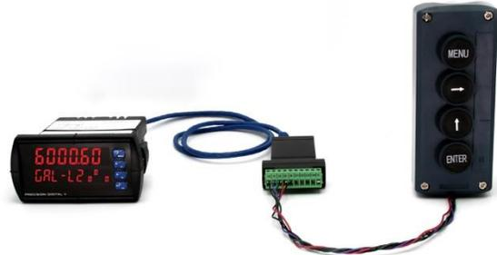
Figure 25. Meter to Control Station Connection
