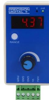
The [PD9502](#) is a low-cost, compact, simple to use 4-20 mA or 0-10 VDC signal generator. It can easily be set for 0-20 mA, 4-20 mA, 0-10 V or 2-10 V ranges. Signal adjustment is made with a one-turn knob. A 15-27 VDC wall plug is provided with the instrument. Optional USB power bank is available.
