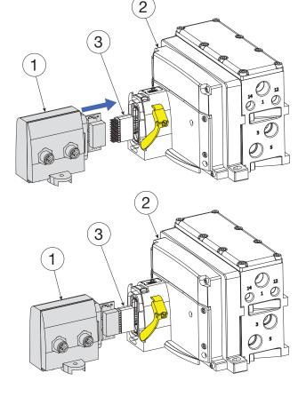
5. Push the P2M Communication Node (Item 1) fully into the H Universal left endplate.
