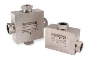
Parker Autoclave Engineers Medium Pressure fittings, nicknamed "Slimline SF", are designed for use with SM Series valves and Parker Autoclave Engineers' Medium Pressure tubing. They incorporate conedand-threaded connections with the orifice sized to match the high-flow 15,000 psi tubing options shown later in this brochure. For instructions on how to make this Medium Pressure Cone & Thread connection and the tools necessary to accomplish, see our "Tools and Installation" brochure.
