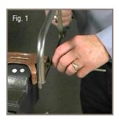
Additional 1/16" should be added to each end to compensate for coning/end facing.
