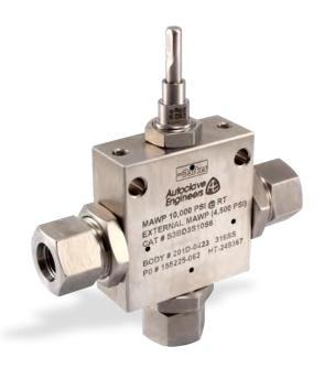
The Parker Autoclave Engineers ball valves can be utilized to switch or isolate flow. The standard material of construction of the valve is 316 cold worked 316/316L with PEEK seats, graphite filled PTFE stem seal, and o-ring material as required by the process fluid.
