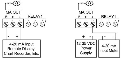
Figure 21. 4-20 mA Output Connections
