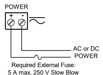
Figure 8. Power Connections
