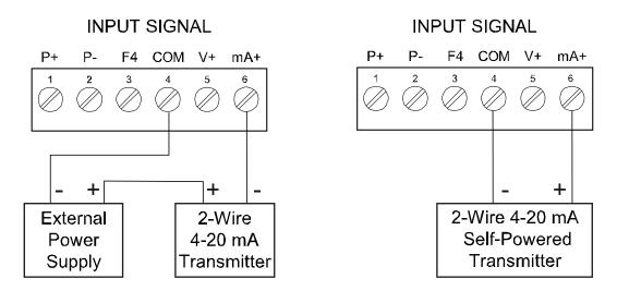
Figure 10. Transmitter Powered by Ext. Supply or Self-Powered
