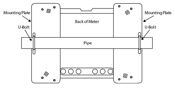
Figure 5. Horizontal Pipe Mount Assembly
