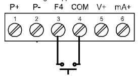
Figure 20. F4 Digital Input Connections
