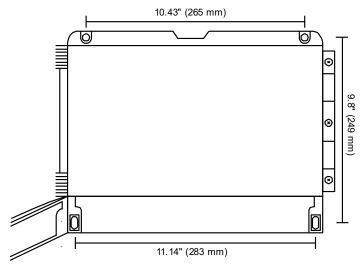
**Figure 1. Meter Mounting Holes**
