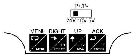
Figure 6. Transmitter Supply Voltage Selection
