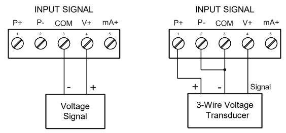
Figure 11. Voltage Input Connections
