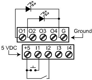
Figure 19. Digital Input and Output Connections
