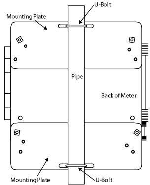
Figure 4. Vertical Pipe Mount Assembly
