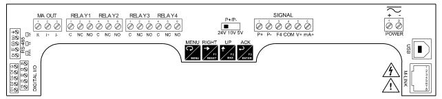
Figure 7. Connector Labeling for Fully Loaded PD2-6200
