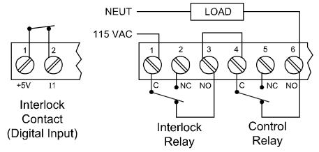
**Figure 22. Interlock Connections**
