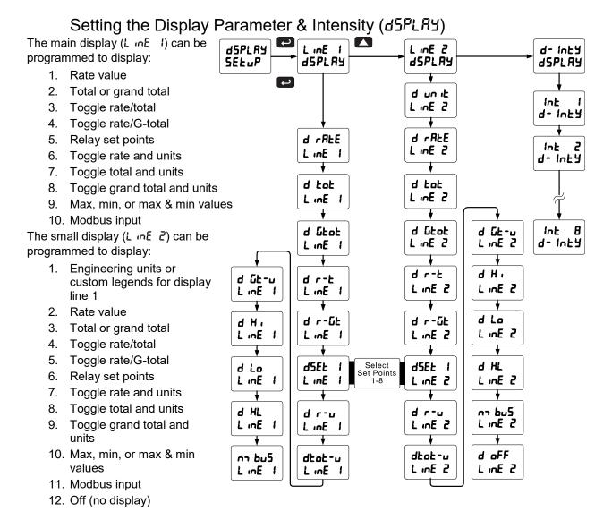
Selecting engineering units or custom legends as display line 2 (d un ib) will display the unit or tag selected for the rate, total, or grand total displayed in display line 1. For example, if line 1 is set to botal selecting d un ib to display on line 2 will have the total appear on line 1, and the total unit appear on line 2
