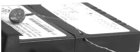
Figure 7. Wire Loop through Rear Case Pass-Through
