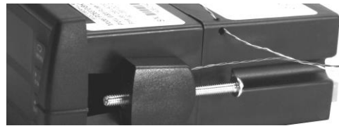
Figure 8. Wire Loop through Security Bracket Pass-Through
