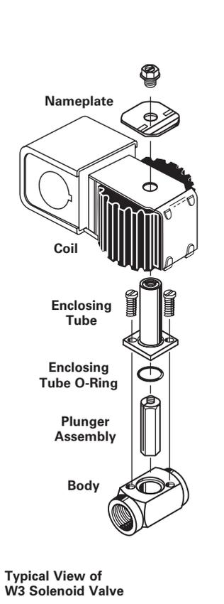
\*B and E Series Solenoid Valves have been redesigned. The new design can be easily identified as a thin, synthetic coated metal gasket, known as a Wolverine gasket. The old gasket is a thicker type of O-ring with a square cross section, known as a tetraseal. See the partial cross sections of the valve body below. The gaskets and the enclosing tubes of the two designs are not interchangeable. The new enclosing tube assembly is included in the replacement parts kits.
