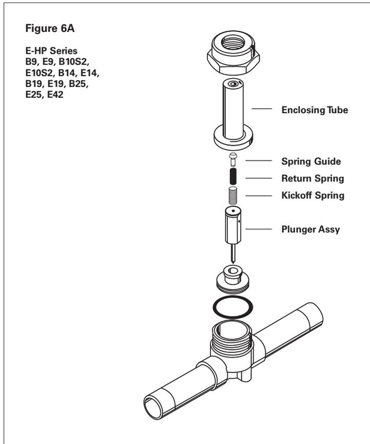
**COILS and INTERNAL PARTS KITS for CURRENT and OBSOLETE VALVE TYPES**
