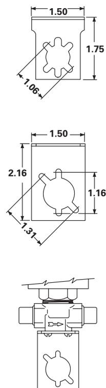
Installation for Types A3, E3\*, E5\*, B6, E6\*, W6, E8\*, B9, E9\*, B10, E10S1\*, E10S2, B14, E14, W14, B19, E19, W19, B25, E25, W25, Series Solenoid Valves.
