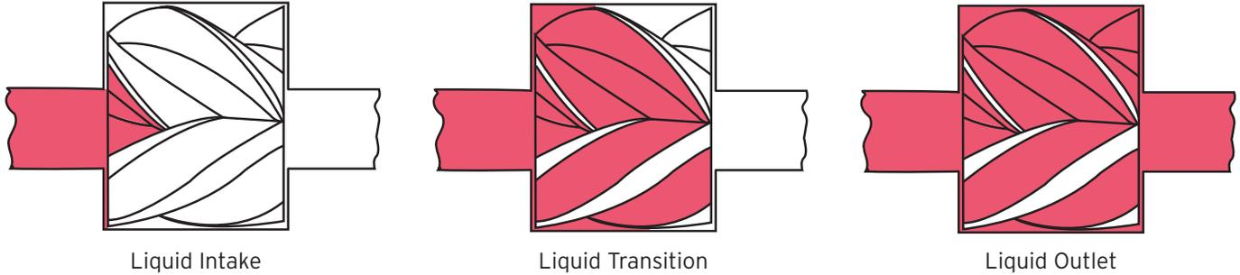
Figure 1- Brodie BiRotor Meter Principle of Operation
