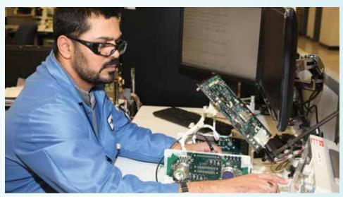
Circuitry for FSD's fuel quantity gauging and management computers is thoroughly tested on in-house-developed equipment to verify correct input and output readings. Our components are tested to exceed all OEM specifications.
