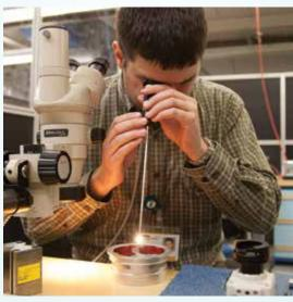
Visual inspections of pump components are crucial after qualification testing to determine if damage or wear is present.
