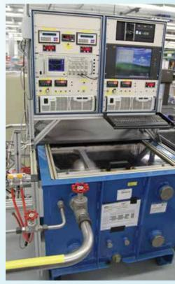
Production test tanks throughout FSD are used to evaluate pumps to document performance characteristics.
