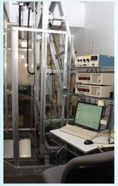
FSD's test stands for in-tank gauging components allow us to simulate a fuel tank environment. Calibration fluid is used to avoid the inherent combustion risks of using fuel.
