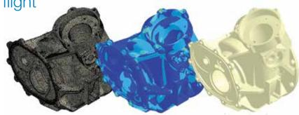
The finite element analysis (FEA) mesh rendering allows the isolation of minuscule elements to calculate stresses in complex geometries.  FEA also helps determine whether the housing has sufficient thickness to withstand various pressures.
