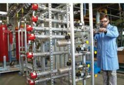
The FSD team puts each ASM design through rigorous test scenarios to meet strict requirements for tolerance and resistance. An endurance test rig is pictured above.
