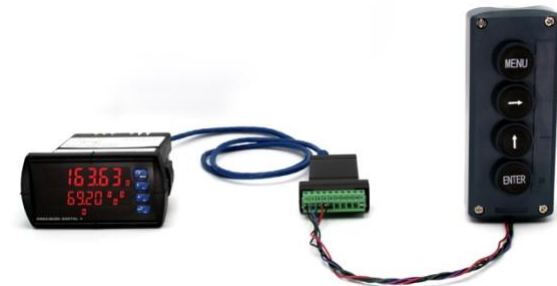
Figure 29. Meter to Control Station Connections
