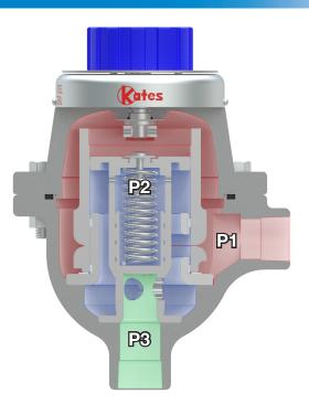
The Kates Automatic Flow Rate Controller combines an adjustable orifice and an internal regulating valve to automatically control flow rate regardless of upstream or downstream pressure variations.
