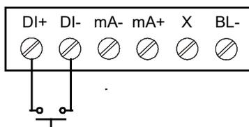
Figure 11. Digital Input Connections
