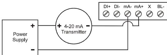
Figure 9. 4-20 mA Input Connection without Backlight
