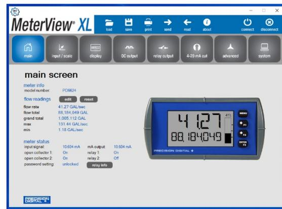
All models come equipped with two open collector outputs and are available with two solid state relays and isolated 4-20 mA analog output options. The open collector outputs are useful for alarm indication or pulse output. The relays can be programmed for alarm indication, on/off control, or pump alternation.
