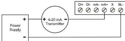
Figure 10. 4-20 mA Input Connection with Backlight
