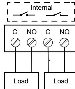
Figure 13. Solid State Relay Connections
