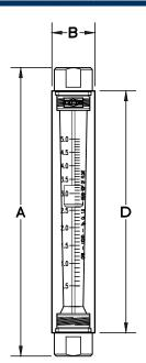
Acrylic block construction with direct reading scales have white screen printed backs to enhance scale readability. Connections are in-line for easy installation.
