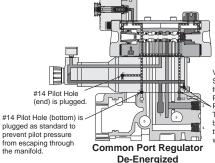
Valve must be set up for External Pilot. Sandwich Regulator configured for External Pilot with the Pilot Plug moved from the bottom #12 Pilot Hole to end #12 Pilot Hole. This allows External Pilot pressure from base to feed through the regulator to the valve without communicating with Main Line Pressure.
