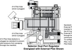
Sandwich Regulator is configured for External Pilot when the Pilot Plugs are inserted into the "P Pilot Holes on both the #12 and #14 ends. This allows External Pilot pressure from base to feed through the regulator to the valve without communicating with Main Line Pressure. To configure the regulator for Internal Pilot, move the Pilot Plugs to the "E" Pilot Holes no both the #12 and #14 ends.
