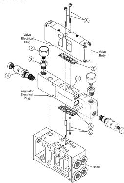
Figure 1 **HB Common Port Sandwich Regulator** (Valve & Base shown for reference only)
