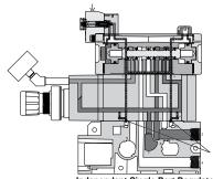
Sandwich Regulator is configured for Internal Pilot when the Pilot Plugs are inserted into the "E" Pilot Holes on both the #12 and #14 ends. This prevents line pressure from escaping through the manifold. To configure the regulator for External Pilot, move the Pilot Plugs to the "I" Pilot Holes on both the #12 and #14 ends.
