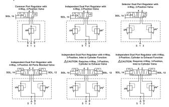
**NOTE:** The Regulators shown on the 14 and 12 End of Independent Port and Selector Units may be replaced with a By-Pass Plate to provide unregulated pressure.
