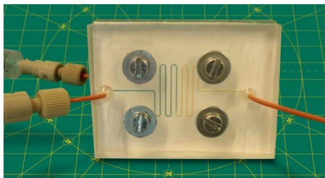
Micro reactor used for testing the CO<sub>2</sub>-permeability of membranes (source: University of Twente, NL)
