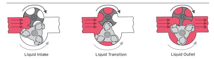
Figure 1 - BiRotor Meter Principle of Operation Diagram
