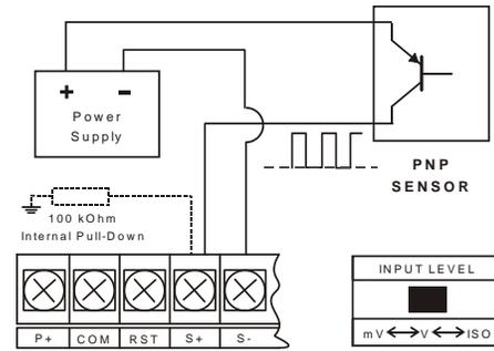
Figure 6. PNP Sensor with External Power (PNP)
