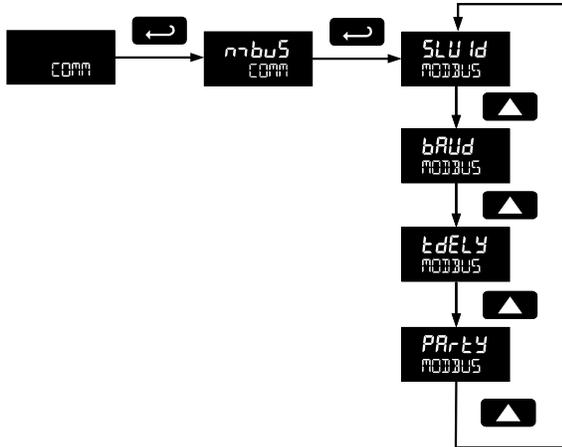
Modbus communications is performed with the 2-wire RS-485 with Modbus RTU option.
