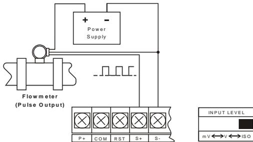
Figure 3. Isolated Flowmeter Powered by External Supply (ISO)
