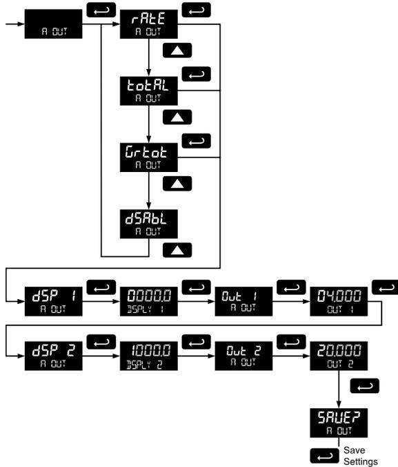
**CAUTION** Please note that when power is removed from the meter, the analog output will drop below 1 mA. Take this effect into consideration when designing any system using the 4-20 mA output.
