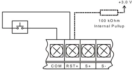
Figure 9. Reset Connections
