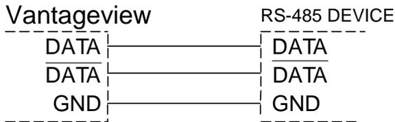
Figure 11. RS-485 2 Wire Serial Connections
