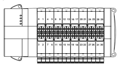
Addressing : Double and single address subbases mixed
