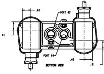
5/2, 4-Way 2 Position Dual Solenoid Port Identification: 1- Pressure/2, 4 - Cylinder/3, 5 - Exhaust
