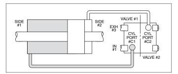
Both coils energized. The inlet pressure is open to side #1 of the cylinder through cylinder port #C1 and the exhaust is closed off. Side #2 of the cylinder is open to the exhaust through cylinder port #C2 and the inlet pressure is closed off by the plunger insert. The piston moves to the right.
