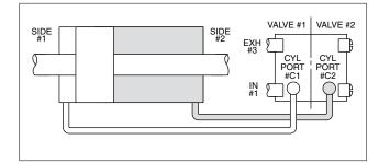
Coil of valve #1 energized; coil of valve #2 de-energized. The inlet pressure is open to side #1 of the double-acting cylinder through cylinder port #C1, the exhaust is closed off by the plunger insert. Side #2 of the cylinder is open to exhaust through cylinder port #C2, the inlet is closed off by the plunger insert. The piston moves to the right.
