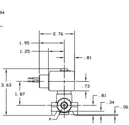
4-Way 2 position single solenoid Port identification: de-energized: pressure to A B to exhaust energized: pressure to B A to exhaust
