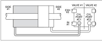
Coil of valve #1 de-energized; coil of valve #1 energized. The inlet pressure is closed off to side #1 of the double-acting cylinder; the exhaust is open through cylinder port #C1. Side #2 of the cylinder is closed to the exhaust and open to inlet pressure through cylinder port #C2. The piston moves to the left.
