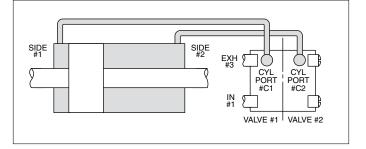
Coil of valve #1 energized; coil of valve #2 de-energized. The inlet pressure is closed to side #1 of the double-acting cylinder and open to exhaust through cylinder port #C1. Side #2 of the cylinder is open to the inlet pressure, through cylinder port #C2. The exhaust is closed off by the plunger insert. The piston moves to the left.
