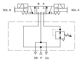
Independent Port Regulator with 4-way, 3-position, All Ports Blocked Valve
