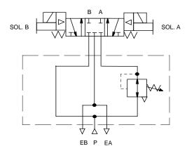
Independent Port Regulator with 4-way, 3-position, All Ports Blocked Valve
