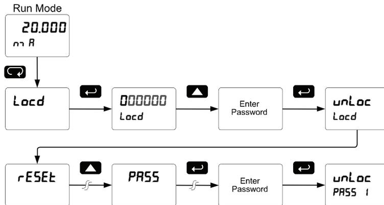
If the correct six-digit password is entered, the controller displays the message *unLoc* (unlocked) and the protection is disabled until a new password is programmed.
