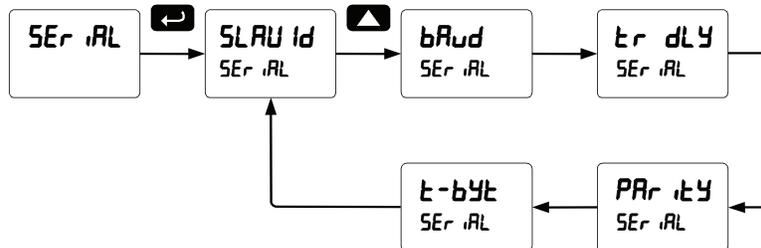
When using more than one controller in a multi-drop mode, each controller must be provided with its own unique address. The controller address (Slave ID) may be programmed between 1 and 247. The transmit delay may be set between 0 and 199 ms. The parity can be set to even, odd, or none with 1 or 2 stop bits.
