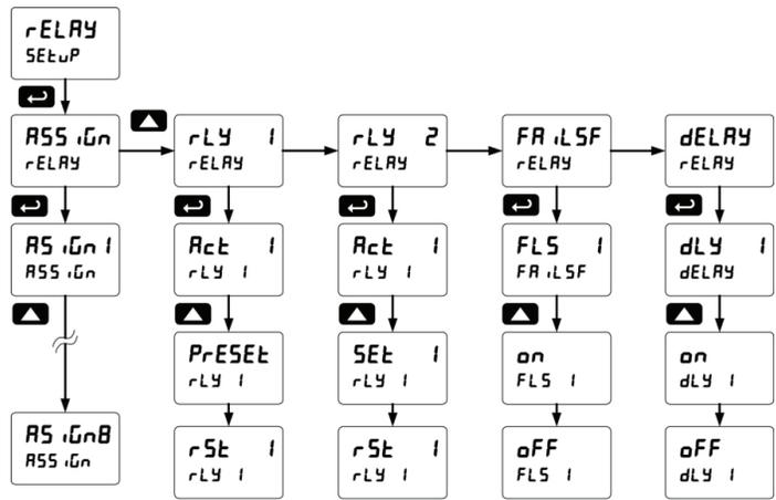
Note: The setup of relays 3-8 follows the same pattern shown here for relay 2.
