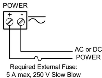
**Figure 6: Power Connections**
