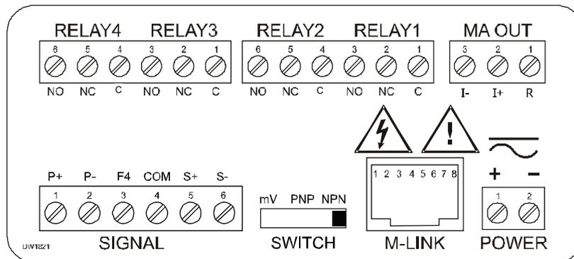
**Figure 5: Connector Labeling for Fully Loaded PD6310**
