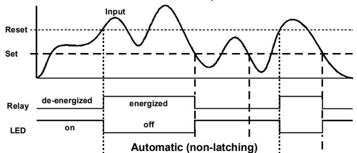
*Note: Relay coil is energized in non-alarm condition. In case of power failure, relay will go to alarm state.*
