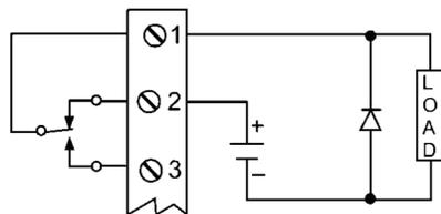
Use a diode with a reverse breakdown voltage two to three times the circuit voltage and forward current at least as large as the load current.
