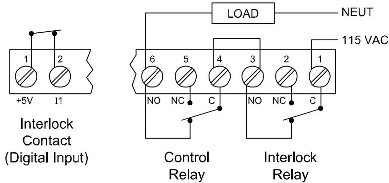
**Figure 21: Interlock Connection**
