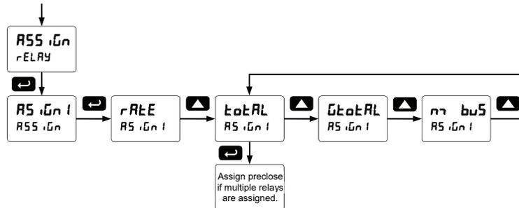
*Note: Relay 1 should always be assigned to “total” for batch control applications.*
