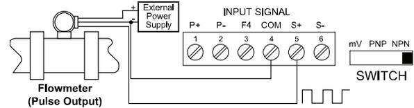
**Figure 8: Flowmeter Powered by External Supply**
