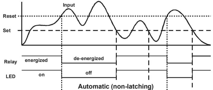
**High Alarm with Fail-Safe Operation (Set > Reset)**
