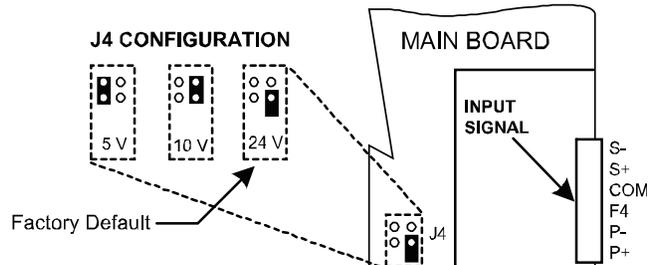
**Figure 4: Transmitter Supply Voltage Selection**
