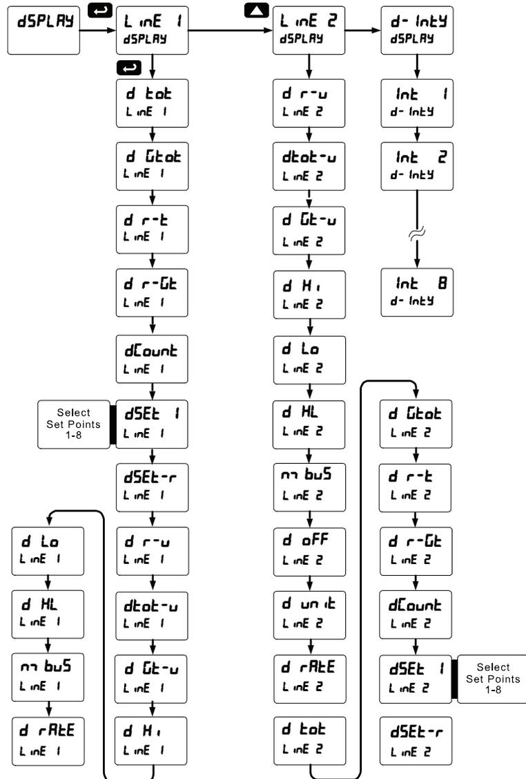
Display Intensity: The meter has eight display intensity levels to give the best performance under various lighting conditions. Select intensity 8 for outdoor applications. The default intensity setting is 8.
