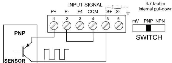
**Figure 11: PNP Sensor Powered by Internal Supply**
