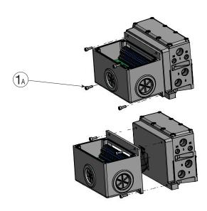
Remove 10 pin and 30 pin connectors from the terminal board
