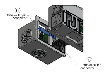
3. Remove (4) M4 screws (Item 1B) that are used to attach the PCB into the box and slide the board out of the box
