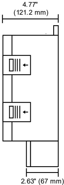
Figure 2. Meter Dimensions - Side View
