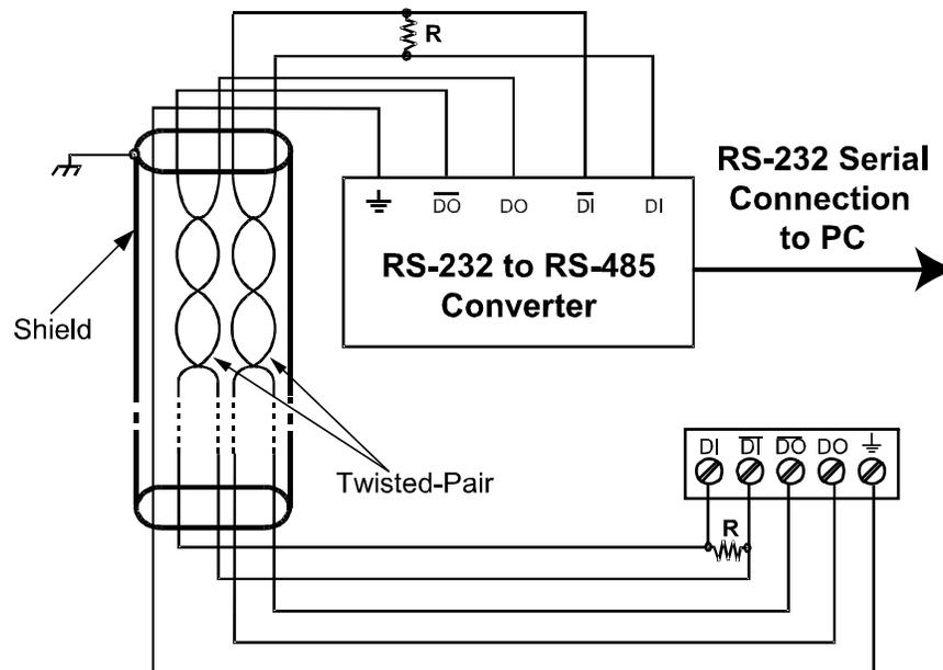
**Figure 10. RS-422 or RS-485 Wiring**
