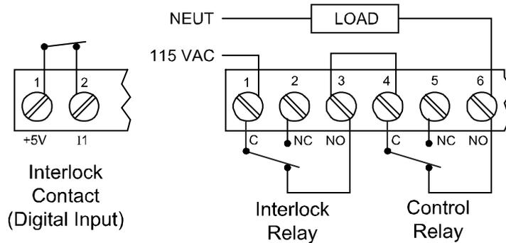
**Figure 20. Interlock Connections**
