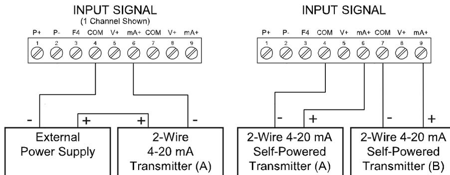
**Figure 22. Transmitter Powered by Ext. Supply or Self-Powered**
