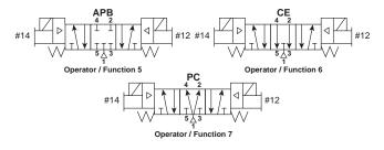
With #12 operator energized – inlet port 1 connected to cylinder port 2, cylinder port 4 connected to exhaust port 5.
