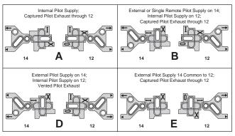
PJLP02 Manifolds can be used for External Pilot, NOT Remote Pilot
