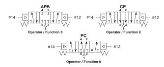
With #12 operator signaled – inlet port 1 connected to cylinder port 2, cylinder port 4 connected to exhaust port 5.
