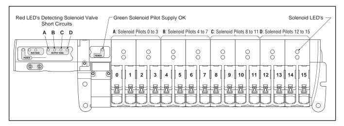
Inside the communication module, solenoid valve control is protected against short-circuits with the following visual indication provided:
