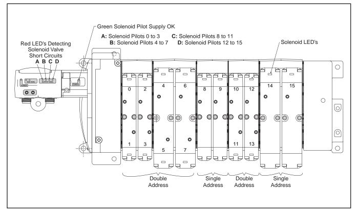
Inside the communication module, solenoid valve control is protected against short-circuits with the following visual indication provided:
