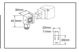
Note: Max ø6.5mm cable size required for connector w/o 6' (2m) cord. IP65 rated when properly installed.
