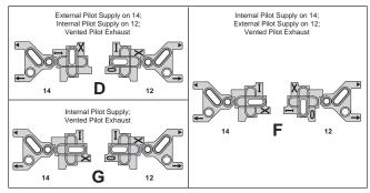
A plug may be inserted in the EXH Port of the PEJ02 & PEJ01 Manifold End Plates, #12 of PL02 & PL01 Subbases.
