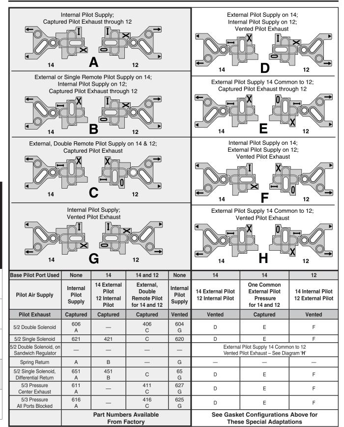
Insert a muffler or vent in the EXH Port of the PEJ02 & PEJ01 Manifold End Plates or #12 of PL02 & PL01 Subbases when using solenoids with a Captured Exhaust.
