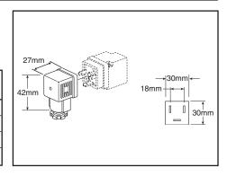
Note: Max ø6.5mm cable size required for connector w/o 6' (2m) cord. IP65 rated when properly installed.
