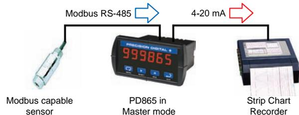
The Snooper can be equipped with a 4-20 mA output option which will convert the serial input to the Snooper into an isolated 4-20 mA output.
