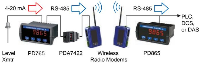
The Snooper can be connected to the Modbus serial output from devices like digital panel meters, temperature controllers, flow indicators, etc to provide indication of the process at another location. The advantage of going digital, is both indicators always read the same value. If an analog output is used, the two displays often read different values.
