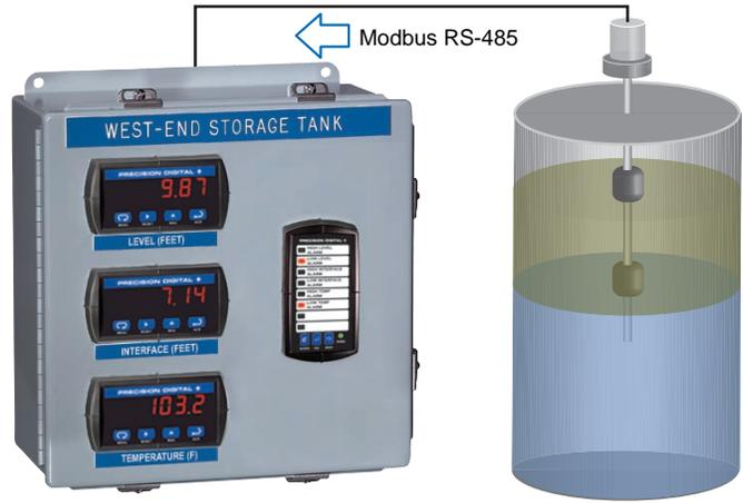
The top Snooper is displaying product level and it is set up as a master device to the level transmitter's slave device. The next two Snoopers are set up in Snooper mode and they are displaying interface and product temperature. Each Snooper's two relays are connected to the PD158 annunciator to indicate alarm conditions.
