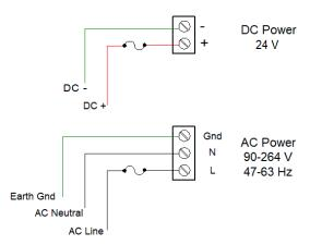
Figure 6. Power Connections
