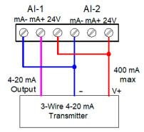
Figure 15. Two Supplies in Parallel Powering 3-Wire Transmitter
