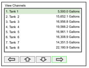
Select any channel using the **Up** or **Down Arrow** keys and Press the **Right Arrow** key again to step into viewing the channel details.
