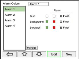
The *Alarm Colors* menu is used to select the colors and behavior of the alarms' text, alarm panel background, and the bargraph indicator for set and reset points.
