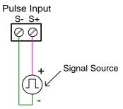
Figure 10. Flow Meter Pulse Input Connections
