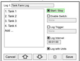
The log *Start / Stop* is used to give the system or the operator control to start and stop the log process.
