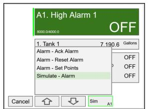
Press the Simulate key to simulate an alarm condition.
