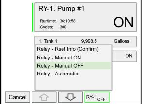
Press the **Manual OFF** to turn off relay 1; Pump #1 will go off and remain off until the relay 1 is put back in automatic mode.
