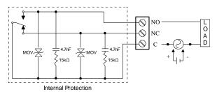
Figure 18. AC and DC Internal Inductive Loads
