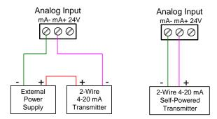
Figure 8. Transmitter Powered by Ext. Supply or Self-Powered
