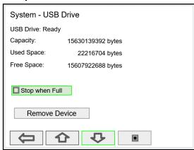
The System – USB Drive provides status information about the connected flash drive.
