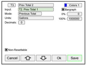
Multiple previous totals can be saved by using a previous total as the input for a new total. Link previous totals to maintain a history of total resets.
