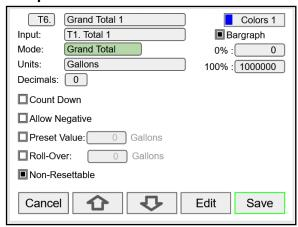
The grand total takes the input from another total and it is not affected by resets of the input total. It is normally set up as non-resettable.
