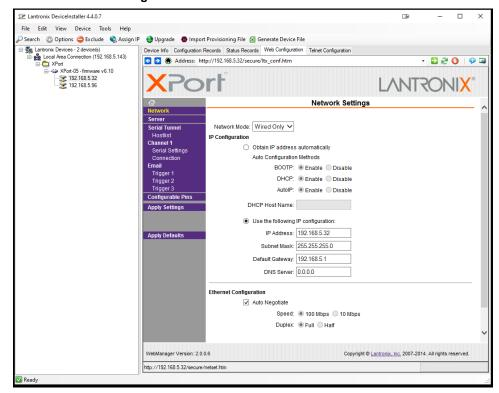
8. Click on Network to assign a new IP Address
