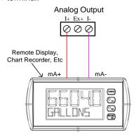
Figure 12. Active 4-20 mA Output Powered by Controller
