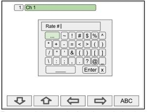
To enter symbols, press the **three dots** and select the desired symbol.
