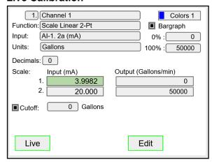
The *Live Calibration* feature is used to calibrate a channel by applying a live calibration signal.
