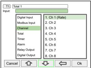
Select the rate input channel for the total and press Ok.
