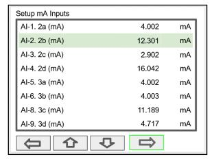
The top line, for each input, shows the slot # and input location (2b = slot #2, second input from the left). It also shows the actual current input.
