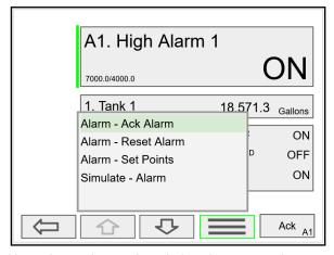
Alarm view options: acknowledge alarm, reset alarm, change set/reset points, and simulate an alarm condition.
