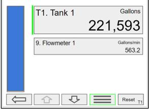
Press the **3-Bar** key to enter a new total, reset the total, or simulate a value for the total.
