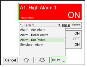
Press the **Set Point** key to change the Set Points. This re-initializes the alarm to reflect the new set point.
