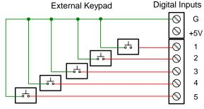
Figure 21. External Keypad Connections
