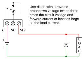
Figure 19. Low Voltage DC Loads Protection
