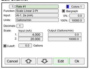
To edit a channel press the **Edit** key and navigate to the setting you want to change, press **Edit** again and make the changes required.
