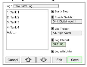
The *Log Interval* can be from 1 sec to 99:59:59 hh:mm:ss. Log entries will be made at the selected interval.
