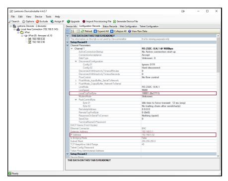
To communicate with a device connected over a LAN, you need the IP Address and the Local TCP Port.
