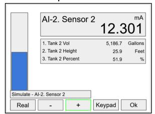
Use the +/- keys to ramp up and down or use the keypad to jump to any value within the range. Press the **Ok** key to maintain the input in simulation mode.
