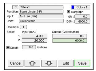
Press the **Save** key to save the changes. The bargraph is automatically adjusted to reflect the scale entered. The bargraph scaling can be changed without affecting the input scaling.
