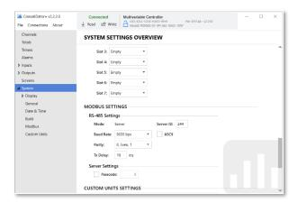
Click on Read, at the top of the screen, to read the configuration of the connected controller. After a read, the channels settings overview is displayed.
