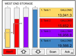
If Alerts are enabled for alarms, the **Menu** key displays a flashing Alert! message on red background.
