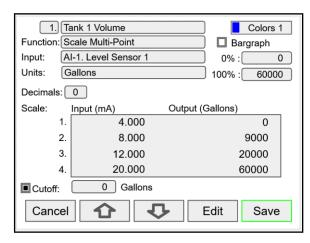
The controller can be configured with up to 50 linearization points. The use of the ConsoliDator+ software is highly recommended for entering the linearization points.
