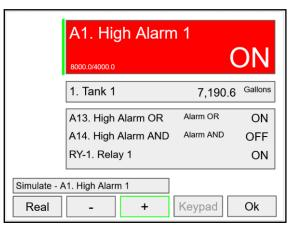
Press the + key to turn on the alarm; note that alarm 13 and relay 1 also turned on. Press **Ok** key to maintain simulation or press **Real** to cancel simulation.
