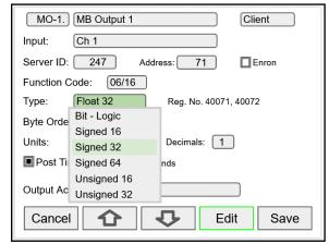
The data type must match the type required by the server device; otherwise the value will not be correct.
