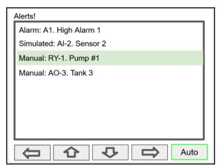
The Alerts! Screen allows the user to acknowledge alarms, return outputs to automatic mode, and navigate to any of the listed items to view the details.
