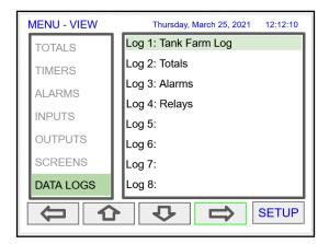
This screens shows a snapshot of the log in progress. If the log is not running, the screen will only show the log # and name. Press *Start Log* followed by *Log Entry* to capture the first log.
