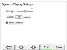
The *Display Settings* menu is used to adjust the backlight brightness, refresh rate and to enable or disable the display of commas for all numeric values.
