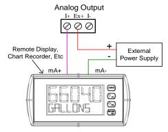
Figure 13. Passive 4-20 mA Output Powered by External Supply
