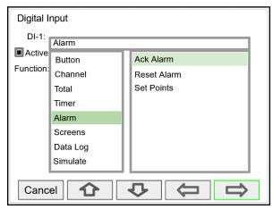
The available functions depend on the I/O cards installed, the Add-On features enabled, and the controller's configuration.
