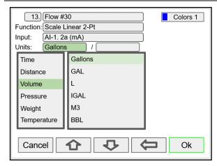
Select the engineering units, decimal point, enter scale points and press the  ${\bf Ok}$  key.
