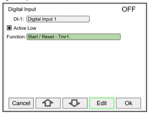
A digital input can be used to execute one of the listed functions and at the same time, it can be used to trigger an alarm or to totalize (count) how many times the function has been executed (e.g. Reset Total).
