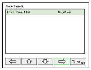
Press the Right Arrow key to step into viewing timer.
