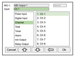
Select the input to be used for the Modbus Output
