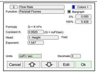
Enter the constant K (for Q = cuFt/sec), the channel used for measuring the head height and the specified exponent. Select the flow rate units. The Controller calculates the flow rate in the specified engineering units. The units can be changed at any time without making any other changes.
