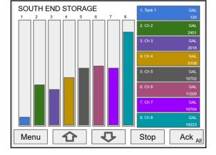
Typical screen view displaying 4 channels and 4 bargraphs representing the values of each channel.
