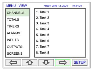
Press the **Right Arrow** key to step into viewing any channel.
