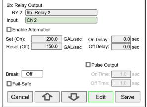
Relays not assigned to alarms are used for automatic on/off control based on set & reset point; they cannot be acknowledged.
