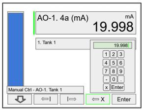
Use the keypad to enter a value for the analog output or use the +/- keys to ramp up and down is small steps.
