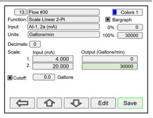
Select number of decimals, scale the input, enter the cutoff value, select colors for bargraph and text, confirm the bargraph's scale, and press **Save**.
