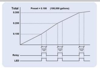
Figure 26. Total Relay Sampling Operation
