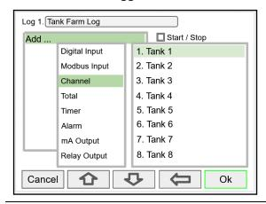
Each log can contain up to 12 process variables, inputs, outputs, timers, alarm status, relay status, or a combination of any of the following parameters:
