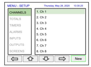
To create a new channel press the **New** key.
