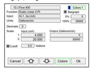
To select a channel color pattern, navigate to the Colors setting and press the **Colors** key.
