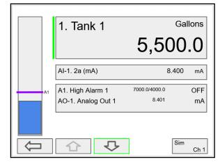
Press the **Down Arrow** key to navigate to the channel input source and then down again to view alarms and analog outputs.
