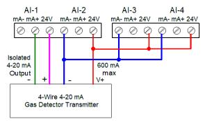
Figure 16. Powering 4-Wire Gas Detector & Isolated 4-20 mA Output
