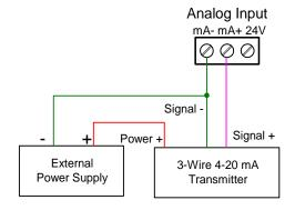
Figure 9. 3-Wire Transmitters Powered Externally
