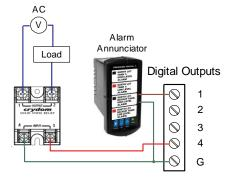
Figure 14. Digital Outputs Driving 5 V Solid State Relay
