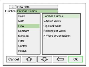
Select the type of weir or flume installed
