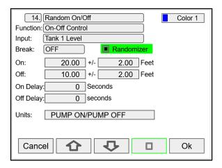
After creating the On-Of Control with Randomizer channel, assign this channel as the input for the relay controlling the pump.
