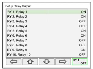
The F4 key can be used to momentarily turn on/off the relays. To manually control the relays, go to the View Menu to set the relay to be permanently on or off.
