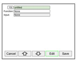
Press the **Edit** key to edit the channel tag and other settings. Press the **Up** and **Down** arrow keys to select setting to be edited.
