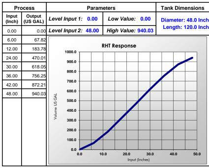
Figure 25. Round Horizontal Tank Volume Graph
