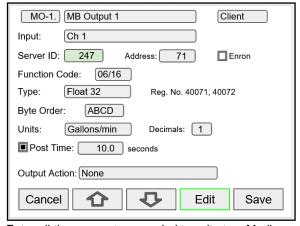
Enter all the parameters needed to write to a Modbus server (e.g. Modbus server panel meter)
