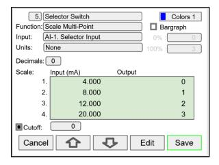
After creating the multi-point channel, assign this channel as the input for the channel with the *Select 1,2,3* function.
