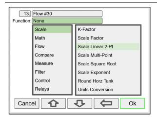
Select the function to be applied to the input and press the  $\mathbf{O}\mathbf{k}$  key.
