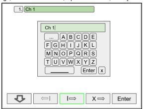
Use the Down Arrow key to navigate to the keypad. Use the |→ and ←| keys to move the cursor and use the X→ key to delete characters. To enter characters in the selected text field, use the **arrow** keys to navigate through the popup keypad.
