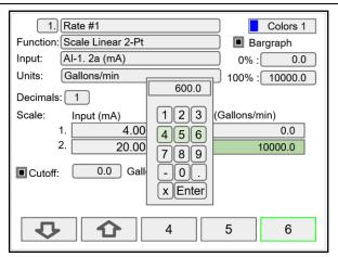
To enter numbers, select the numeric keypad, move the cursor to the insertion point and enter the number using the soft keys.
