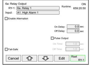
The relay runtime & cycle count can be reset (cleared) from the relay setup screen.
