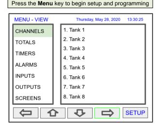
The View screen allows a user to view all the settings and values for Channels, Totals, Timers, etc. To program the instrument, press the **Setup** key.
