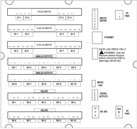
Figure 5. Connection Terminals for a PD9000-GP-4PI-8AI-10AO-10RY
