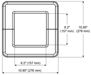
**Figure 1. Front Panel Mount Dimensions**
