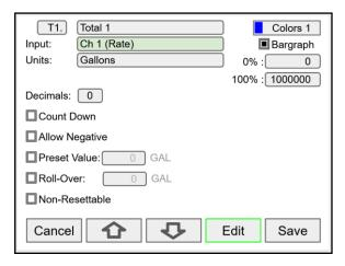
Select total units, count up or down, enter preset and roll-over values, and select non-resettable if required. After pressing **Save**, press **Yes** to reset the total to the preset value.
