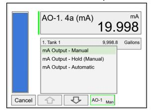
Select **Manual** to control the analog output manually; select **Automatic** to exit manual control.
