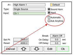
Latching: Acknowledge only after the alarm condition has cleared
