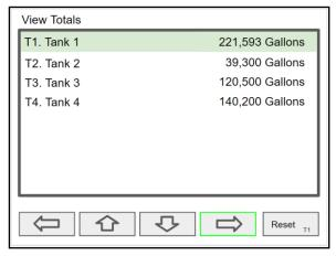
Press **Right Arrow** key to step into details of the selected total and view the source and associated outputs.
