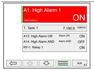
Press the **3-Bar** key to select Ack Alarm, Reset Alarm, change Set Points, or Simulate Alarm condition.
