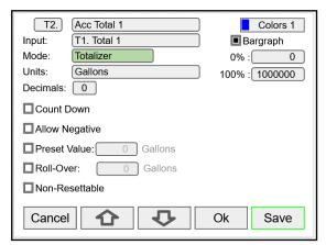
The *Totalizer* mode can be used to add the input total to the new total, when a trigger is activated. The trigger can be a digital input, a Modbus input, or any event selected.
