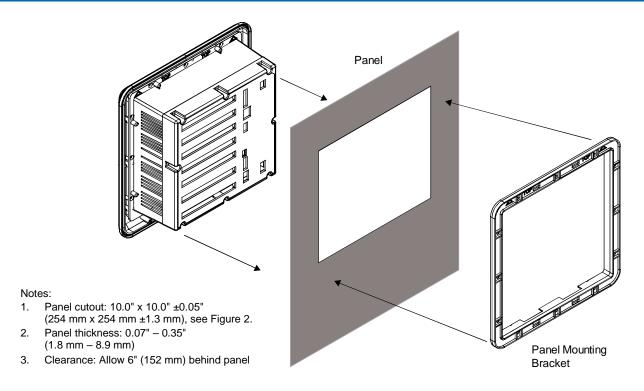
**Figure 3. Panel Mount Installation**
