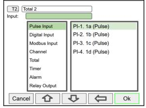
Pulse inputs can be totalized directly without the need to create a rate channel.
