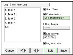
The log *Enable Switch* can be any item with a binary value (on / off, 0 / 1, true / false). Log entries will be made only if the Enable Switch is in the on position.
