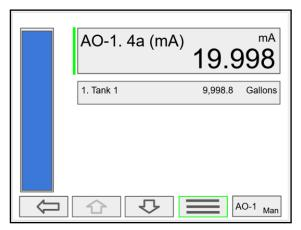
Press the **3-Bar** key to access Analog Output controls. Manual control, hold current value, return to automatic.
