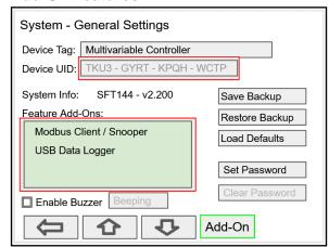
The Add-On Features can be enabled at the factory or they can be purchased and enabled by the user at any time. A unique key code is required to enable Add-On Features.
