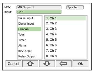
Select the input for Modbus Output.
