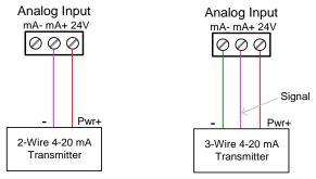
Figure 7. Transmitters Powered by ConsoliDator+
