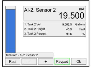
All the parameters associated with the simulated input follow the simulated value. Press the **Real** key to cancel simulation and return to the actual sensor signal.
