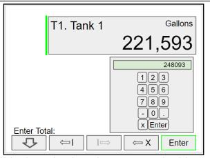
Using the numbers keypad, enter a new total and then press the **Enter** key to save.
