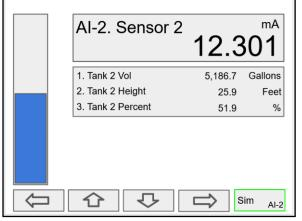
The above screen shows the Analog Input 2 details and the associated channels.
