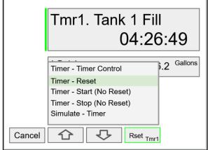
Press the Reset key to reset the timer, select Timer Control for additional functions. Use the Simulate function to simulate the timer rising, falling, or jump to a specific value using the keypad.
