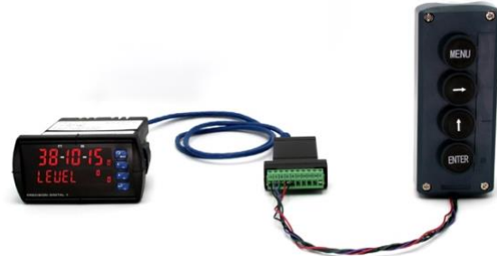
Figure 25. Meter to Control Station Connection
