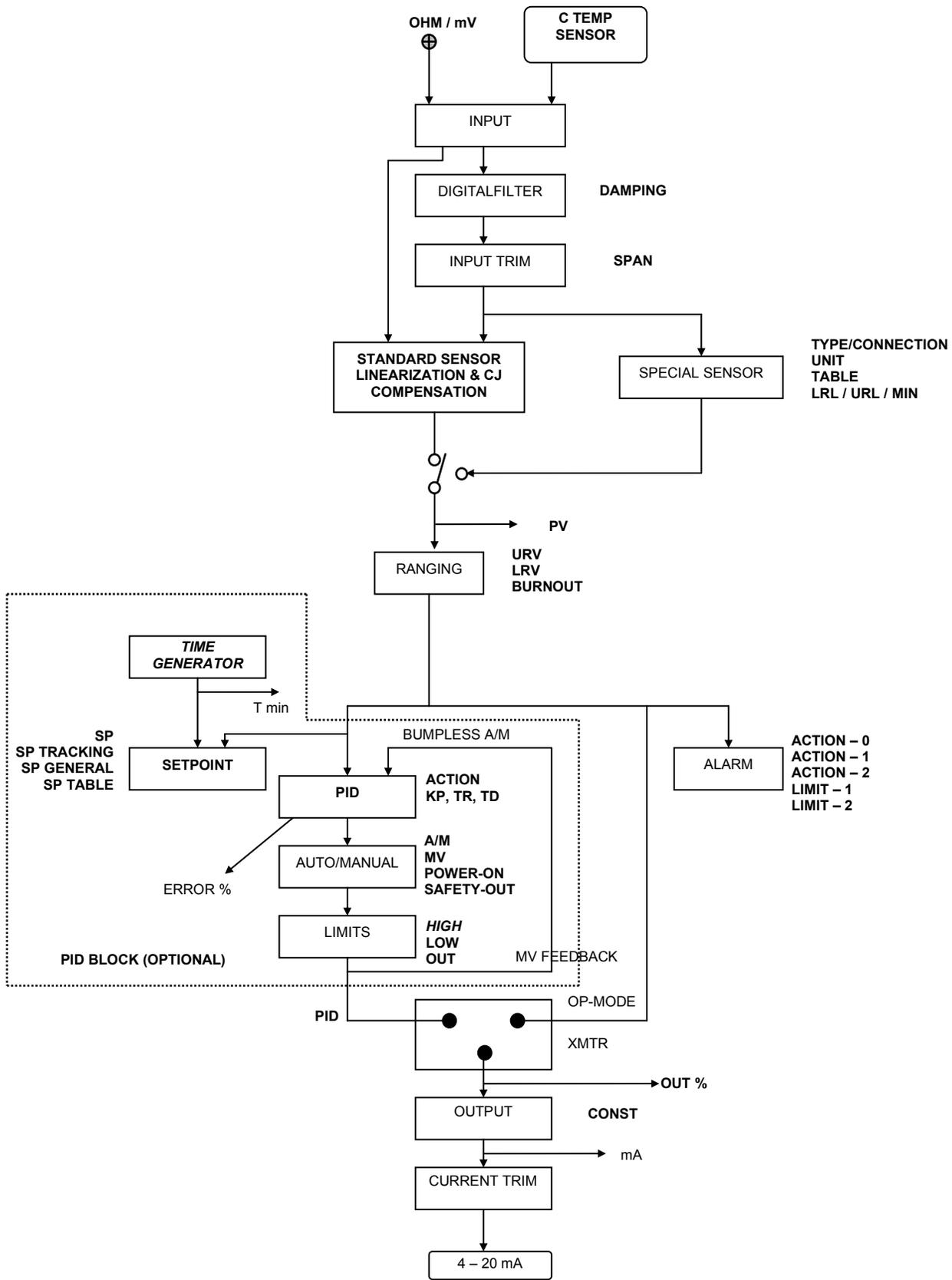
Fig. 2.2 – TT421 Software Function Block Diagram
