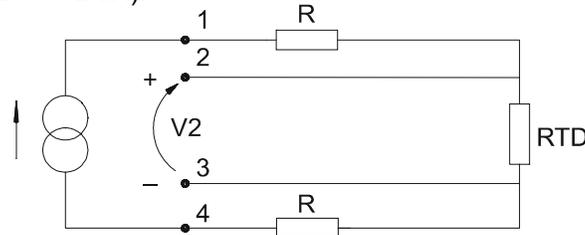
**Fig. 2.5 – Four-Wire Connection**
