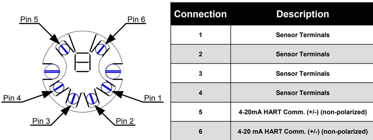
Fig. 1.1 – Connections and description of the TT421.
