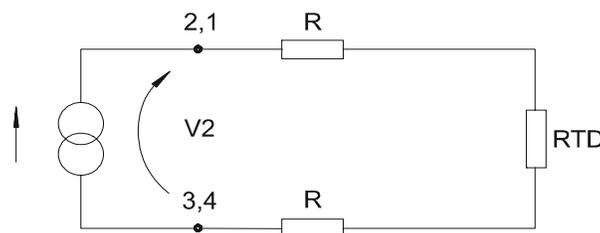
**Fig. 2.3 – Two-Wire Connection**
