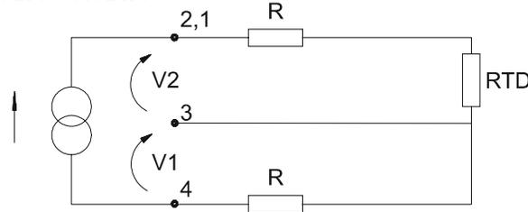
**Fig. 2.4 – Three-Wire Connection**
