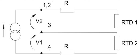
**Fig. 2.6 – Differential Connection**
