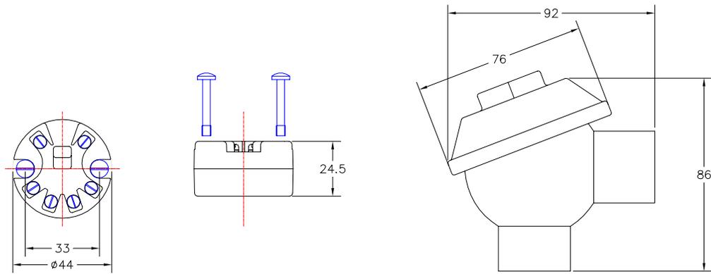
**Fig. 3.7 – Mechanical Dimensions**
