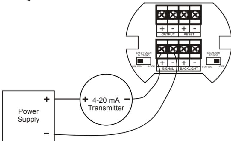
Figure 2. Input Connections without Backlight
