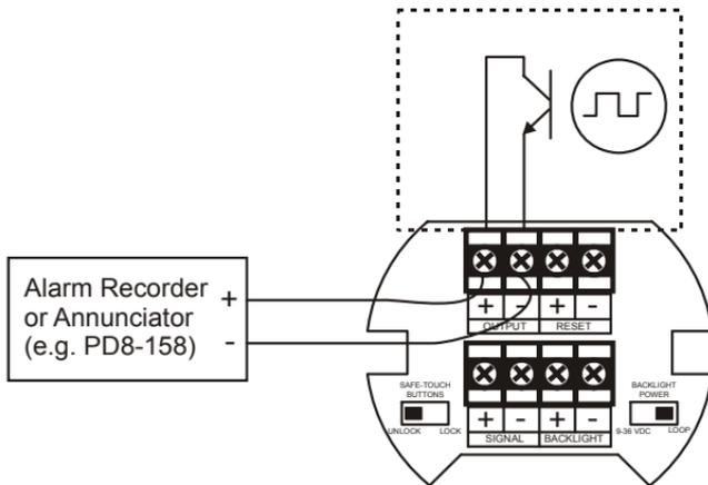
Figure 6. Connection to Device with Internal Pull-Up
