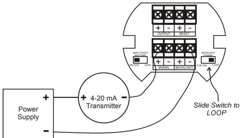
Figure 3. Input Connections with Loop-Powered Backlight
