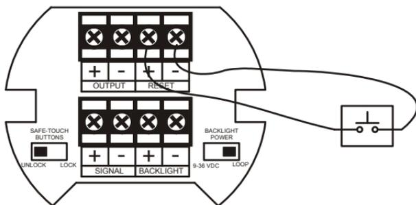
**Figure 5. External Alarm Reset/Acknowledge Connections**
