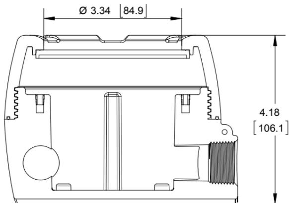
Figure 9. Enclosure Dimensions – Side Cross Section View
