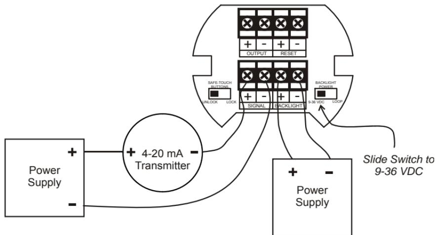
**Figure 4. Input Connections with Externally-Powered Backlight**
