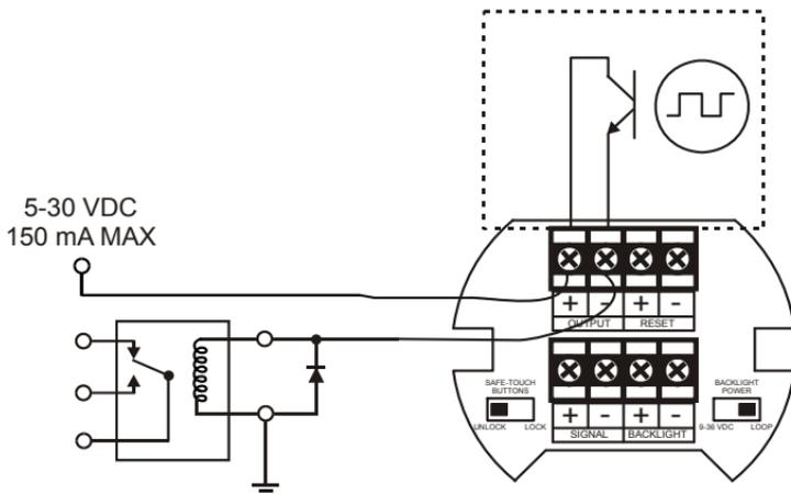
Figure 7. Output Connections
