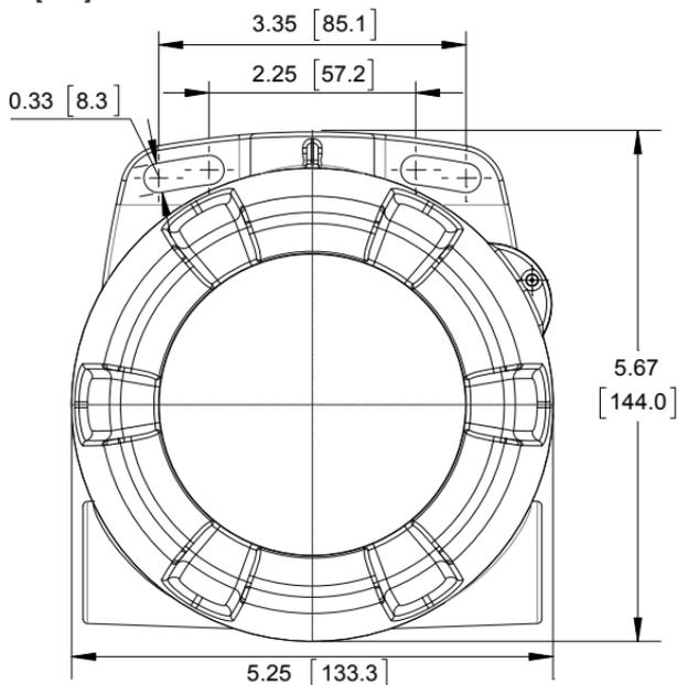
Figure 8. Enclosure Dimensions – Front View
