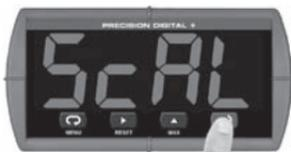
**Note:** The meter will use an internally calibrated signal source to scale the analog output signal. There is no need for a calibrated signal source to scale the analog output.
