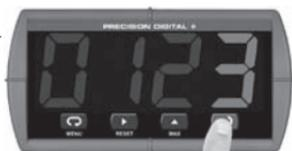
**Note:** In order to unlock the meter once it has been locked, repeat these steps and enter the password. This will remove the password and allow programming of the meter. For more information, please consult the instruction manual.
