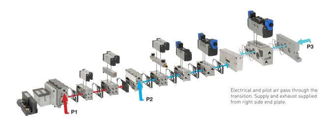
**Pressure Zoning** Multiple Pressure Zones (P1 P2 ... Pn) provide flexibility to meet a variety of applications. Supplying the valves on the manifold with different pressures will allow for variable force output from any attached actuators. In addition, you can control vacuum and remove supply pressure from certain sections while leaving other areas operable. This can be useful in safety applications as well as for maintenance.
