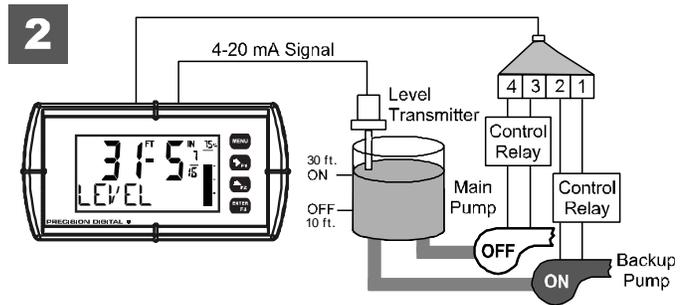
3. If the backup pump is not able to keep up, and the level reaches 40 ft., relay #2 transfers and starts the main pump as well.
