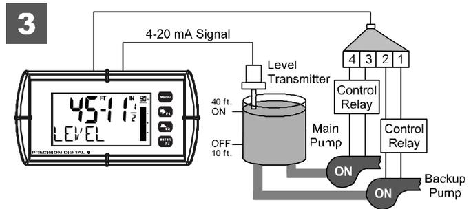
4. Once the level has dropped below the reset points, both relays will turn off.
