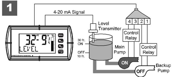
2. With the Pump Alternation feature activated, the next time the level reaches 30 ft., relay #1 transfers and starts the backup pump.
