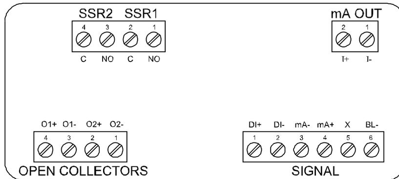
**Figure 4. Connector Labeling for Fully Loaded Meter**
