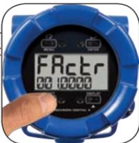
**Note:** The number entered during step 7 is the K-Factor assigned to your specific flowmeter. This number is notated on the flowmeter itself or somewhere in the instruction manual included with the flowmeter. This number is necessary in order to tell the ProtEX meter how many pulses it will receive depending on the flow rate.
