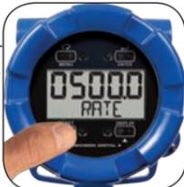
**Note:** Programming the *set point* to be **greater** than the *reset point* will result in a high alarm (meaning the alarm will turn on when the value is greater than the set point). Programming the *set point* to be **less** than the *reset point* will result in a low alarm.
