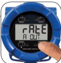
**Note:** The following menus will ask you to program display and output values. A display value is the process value being displayed by the meter. An output value is the current in mA that the meter should output at that display value. Display 1 represents the low end of the display value range while display 2 is the high end. Output 1 is the low end of the analog output and output 2 is the high end.
