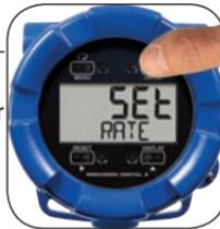
**Note:** This menu will allow you to program the value at which the selected parameter will trigger the alarm. The reset point is the value at which the parameter will deactivate the alarm state.
