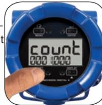
**Note:** The number entered during step 7 is the output pulse count, or the number of pulses that should be outputted per input pulse (adjusted by input K-Factor). For a 1-to-1 ratio, the count should be set to 1. Otherwise, the output will be calculated as follows:
