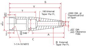
.437" Diameter Tapered Bore, .180" Taper per foot, 1-1/4"-18 NEF2 Internal Thread. For use with Industrials and Cleanliner Thermometers, and Digi-Stem 5/8" diameter with 1-1/4"-18 NEF.
