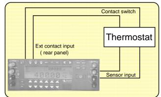
"switch IN" is for a thermostat with a built-in sensor and the INPUT channel of the **Calys 1000/1200** and **Calys 1500** must be connected to a sensor that will read the same temperature of the thermostat and the switch of the thermostat must be connected to a 25-pin connector located on the rear panel of the instrument.
