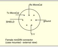
For easy interconnections a miniDIN connector with cable con be supplied on request. The conductors color codes can change with different supplier; please check before using.
