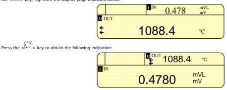
If the  $\langle \bigcirc \rangle$  key is setting for scrolling mode (see par. 8.6), the operator can swap the indication displayed in the upper with the indication in the lower slot by pressing the  $\langle$  shift> +  $\langle \bigcirc \rangle$  keys.
