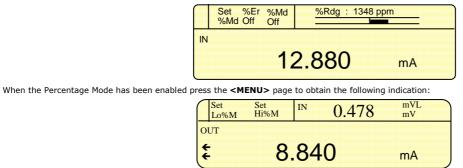
Press one of the above new keys to adjust automatically respectively the 0% value and the 100% value to the actually indicated **IN**put and **OUT**put signal values.
