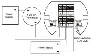
Figure 6. Connections with Externally-Powered Backlight
