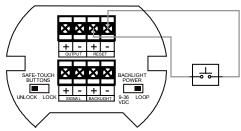
Figure 7. External Alarm Reset/Acknowledge Connections
