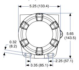
Figure 1. Enclosure Dimensions - Front View
