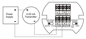
Figure 4. Connections without Backlight
