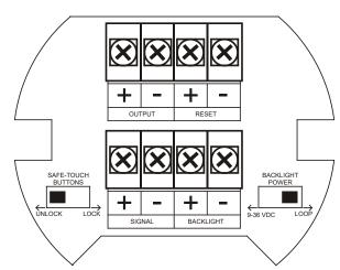
Figure 3. Connector Board
