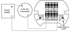
Figure 5. Connections with Loop-Powered Backlight
