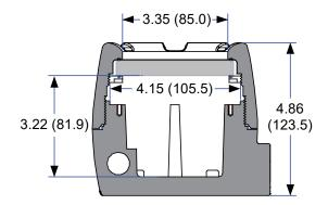
Figure 2. Enclosure Dimensions – Side Cross Section View
