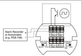
Figure 8. Connection to Device with Internal Pull-Up
